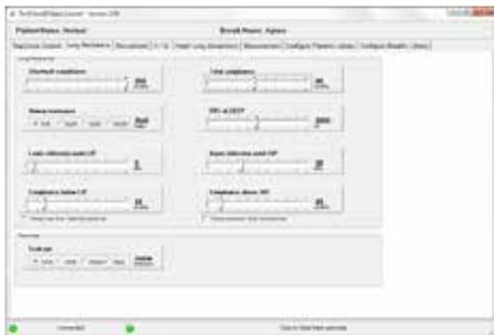
For those who want to influence the parameters directly, Basic Control can access all values that are used in the TestChest physiological model to setup the artificial lung. These include FRC, predicted FRC,
